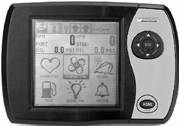
SC5000 System View
